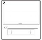
Verify with a level gauge that the inclination of the Soundbar is zero degrees
