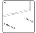
Make the holes with the corresponding drill bit according to the type of wall.
